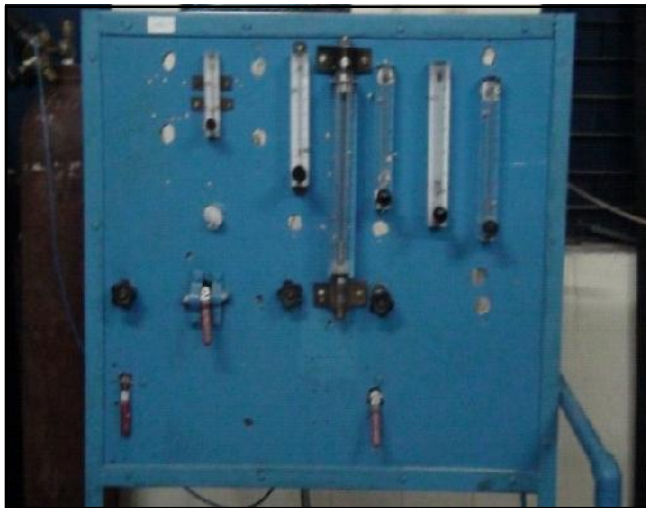
Fig. E : Rota meters for measuring flow rates for hydrogen and air
