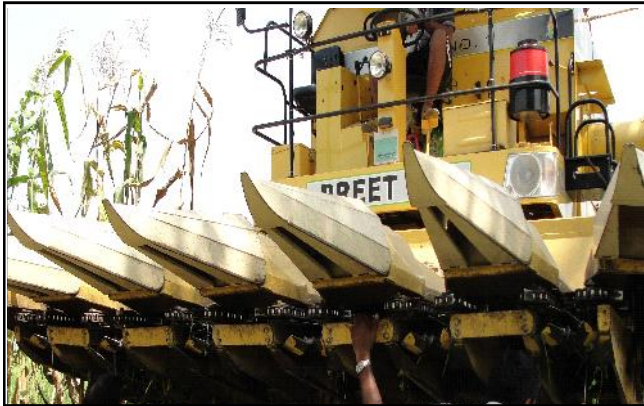
Fig. 1 : Chain conveyor system in snap roll type header maize combine
