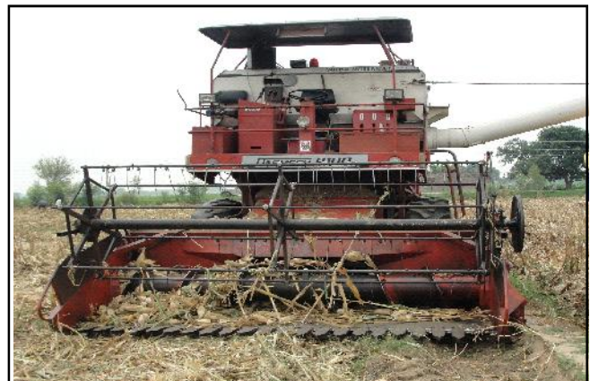
Fig. 3 : Square section reel in cutter bar type header maize combine
