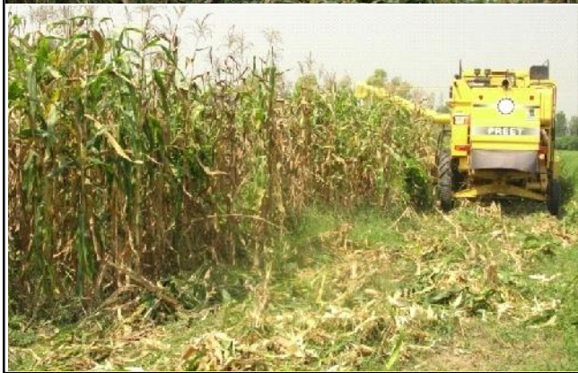
Fig. 2 : Demonstration of maize combine having snap roll type header
