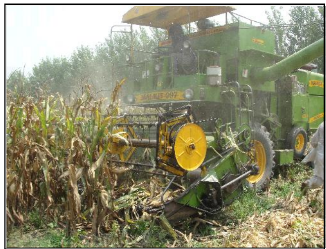
Fig. 4 : Demonstration of maize combine having cutter bar type header
