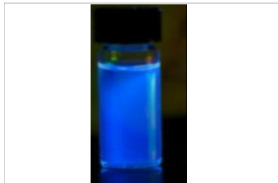
Fig. 4 : Blue luminescence of quantum dots at higher wavelength
